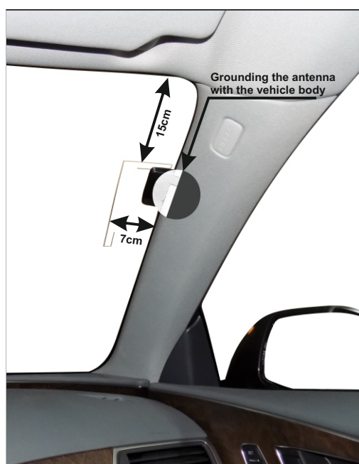
Example of mounting a DAB/DAB+ antenna
