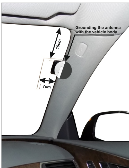
Example of mounting a DAB/DAB+ antenna
