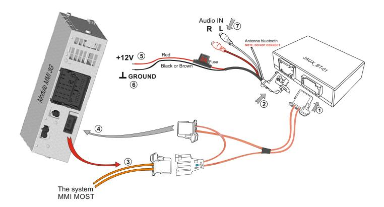
An example of how to connect to a radio module mounted in the trunk compartment
