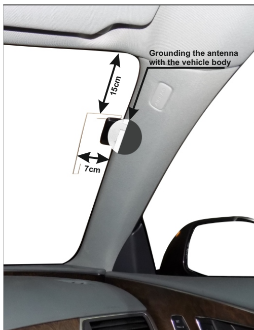
Example of mounting a DAB/DAB+ antenna
