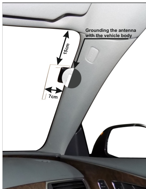
Example of mounting a DAB/DAB+ antenna
